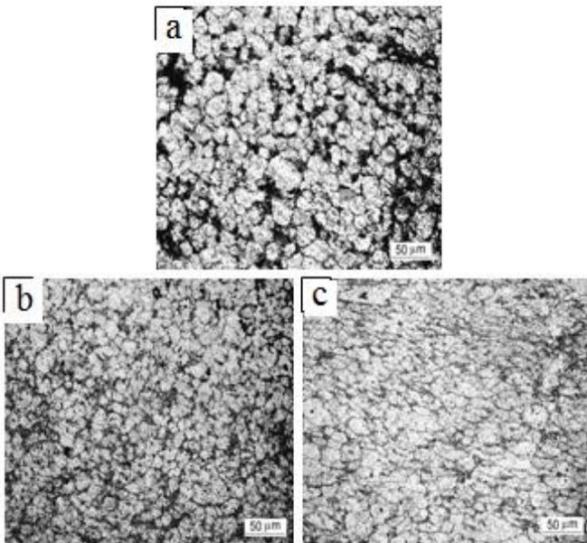
Figure 1: Microstructure of spray deposited Al-6Si-10Pb alloy for (a) 0, (b) 40 and (c) 80 % thickness reduction.
