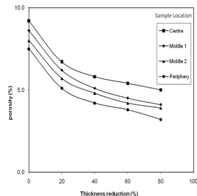
Figure 3: Variation in the porosity of spray deposited Al-6Si-10Pb alloy as a function of thickness reduction at different locations of the preform viz. centre, middle 1, middle 2 & periphery.
