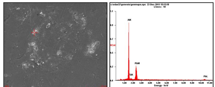
Figure 2: EDS spectrum with analyzed region, indicating Pb and Si phases in spray deposited Al-6Si-10Pb alloy
