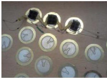
2. Parallel & Series connection of piezoelectric discs
