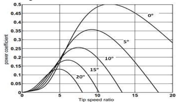
**Figure:-4 Power coefficient Vs Tip Speed Ratio**
