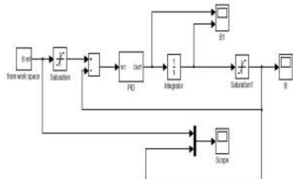
**Figure:-5 Block Diagram with PID controller**
