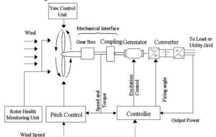
**Figure: 1** General structure of a wind Energy Conversion System Model
