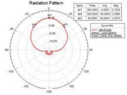
Figure 16. Radiation pattern of antenna array of Fig.5
