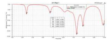
Figure 2. Single rectangular patch S11 (db) graph
