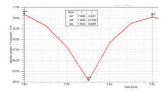
Figure 11. Return loss of antenna array of Fig.3
