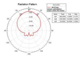
Figure 12. Radiation pattern of antenna array of Fig.3
