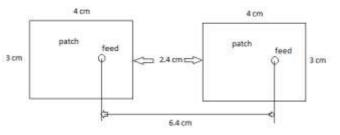
Figure 3. Two element array with feed to feed distance of 6.4 cm
