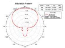
Figure 10. Single microstrip patch antenna radiation pattern
