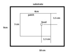
Figure 1. Single rectangular patch with substrate
