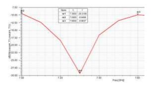
Figure 9. Single microstrip patch antenna return loss
